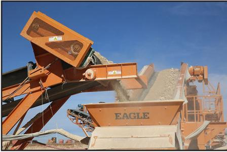
*Integrated 45" feed conveyor remains on for transport and eliminates the need for a separate feed conveyor.*
